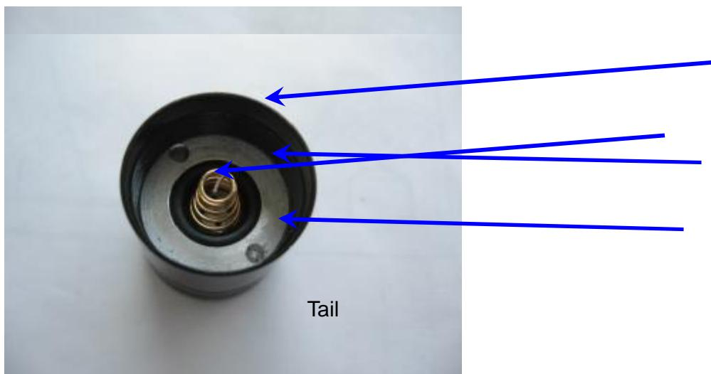
Some Fenix flashlight could not turn on, please use a forceps and insert in both of the two holes inside the tail cap and turn clock wise.
